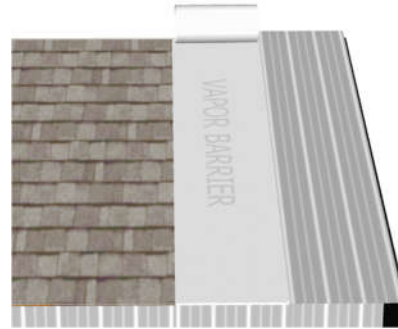
G-Rib over Existing Asphalt (exposed fastener)
