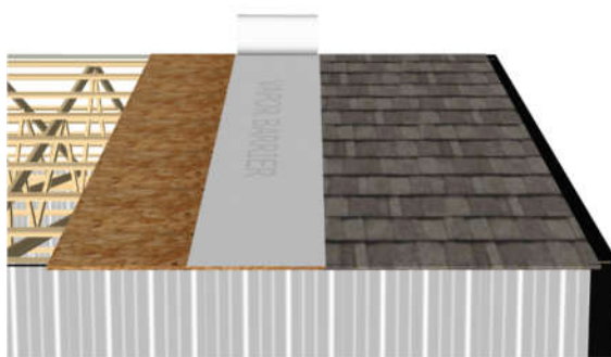
Asphalt Shingle from Owens Corning (hidden fasteners)
